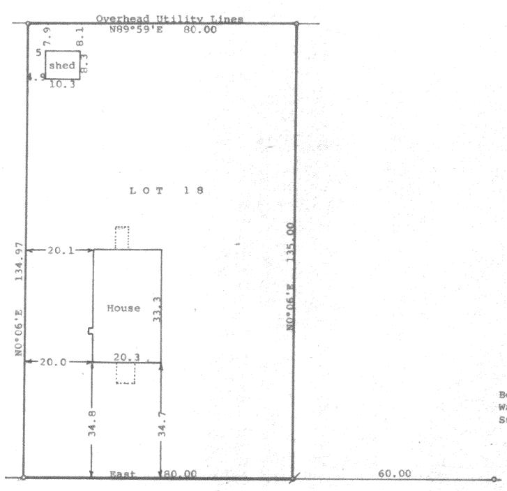
Scale - 1" = 20" • = 1" Iron Pipe Found # = Mark found in subsoil and 3/4° X 24" Iron Pipe Set
